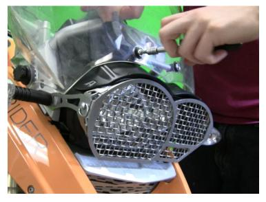
(14) Using a finger to hold the nut in place, and a T-25 torx bit and driver, put the OEM fasteners back that hold the wind screen. Do not forget to tighten the adjustment knobs!
