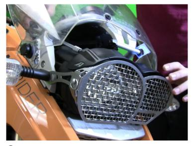
(13) Put the Anti-glare Guard on top of the bezel. Using a T-15 torx bit and an extension, replace the OEM plastic screws with the AltRider provided hardware. Do not overtighten!
