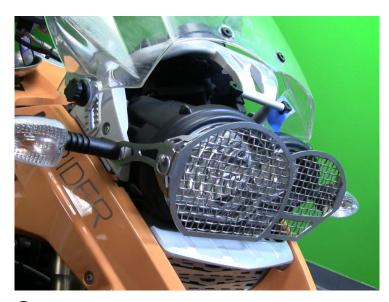
(1) (a) Loosen the two adjustment knobs for the windscreen and (b) rotate the windscreen back so you can access the bezel screws.
