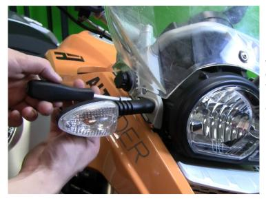
① Using a T-30 torx bit, carefully remove the fastener that secures the turn signal stalk. There is a small nut on the inside of the plastic mount, it can fall out on some bikes!
