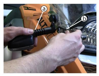
(a) rotate the stalk as shown and push into the stainless arm
