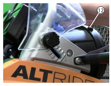
(12) Remove the (2) screws that hold the headlight front bezel. (one on the left and one on the right) Pay attention to the tension of these screws, you will be replacing them.
