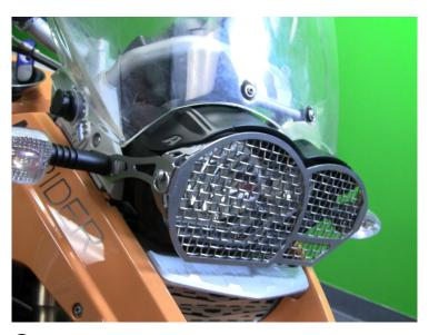
(15) Check to make sure your adjustment knobs, windscreen fasteners and turn signal stalk fasteners are all tightened appropriately.
