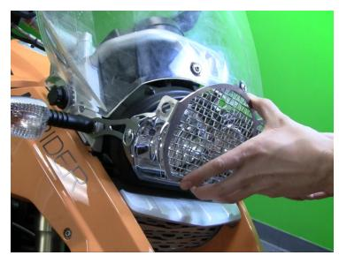
8 Now you can install the headlight guard. First put one side of the guard onto the 1/4-turn fastener without fastening it, then the other side.
