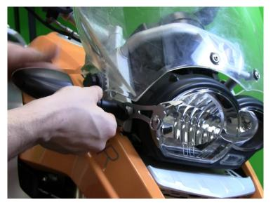
(5) Push the stalk/arm assembly into its place and then rotate the stalk 180 degrees back to its starting position.
