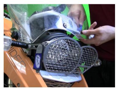
Use a T-25 torx bit to remove the (2) front windscreen fasteners. You can use a little masking tape or a magnetic finger glove to hold the nut on the back side of the windscreen mounts.
