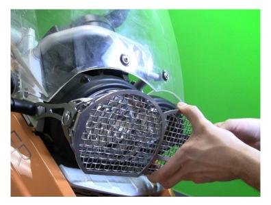
Now you can turn the Dzus fasteners 1/4 turn. If the bike is on its side stand, gravity can make it difficult to engage the fasteners clip. Just hold the clip with your hand while turning.
